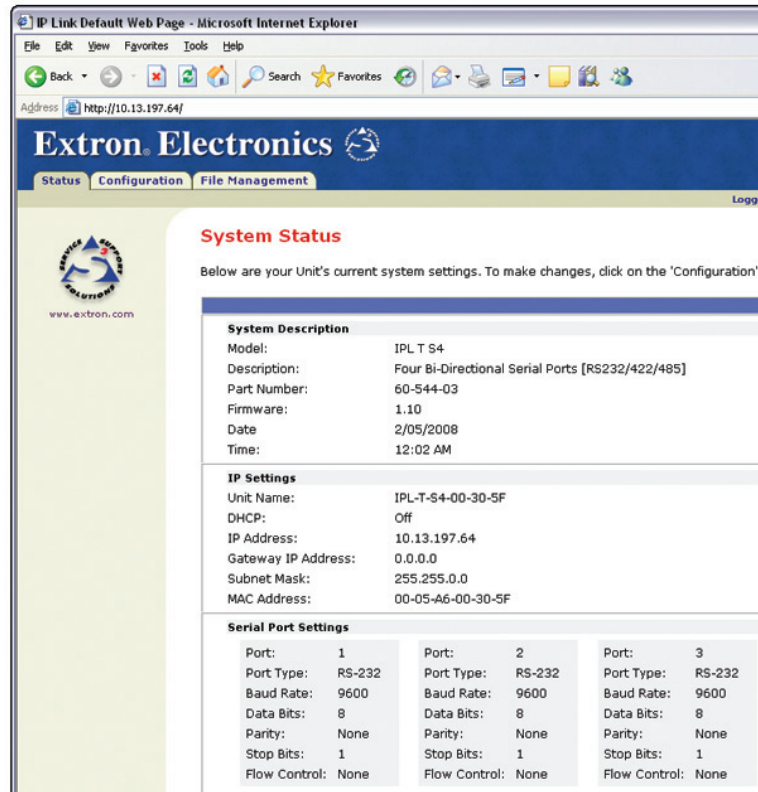
Figure 3-10 — Web server System Status screen
